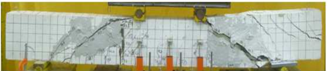
(e) BS-02R (repaired)
