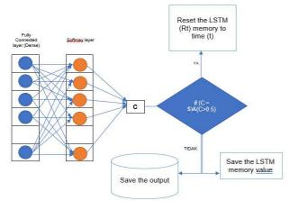
Fig. 5 Modification diagram of output Softmax
