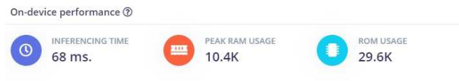
Fig. 9 The total memory usage of the cough detection system developed on Edge Impulse
