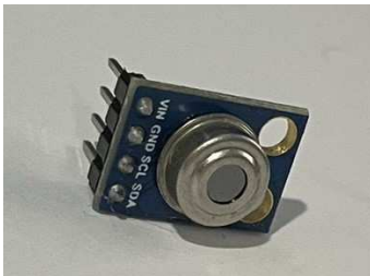
Fig. 3 MLX90614 uses infrared to measure temperature
