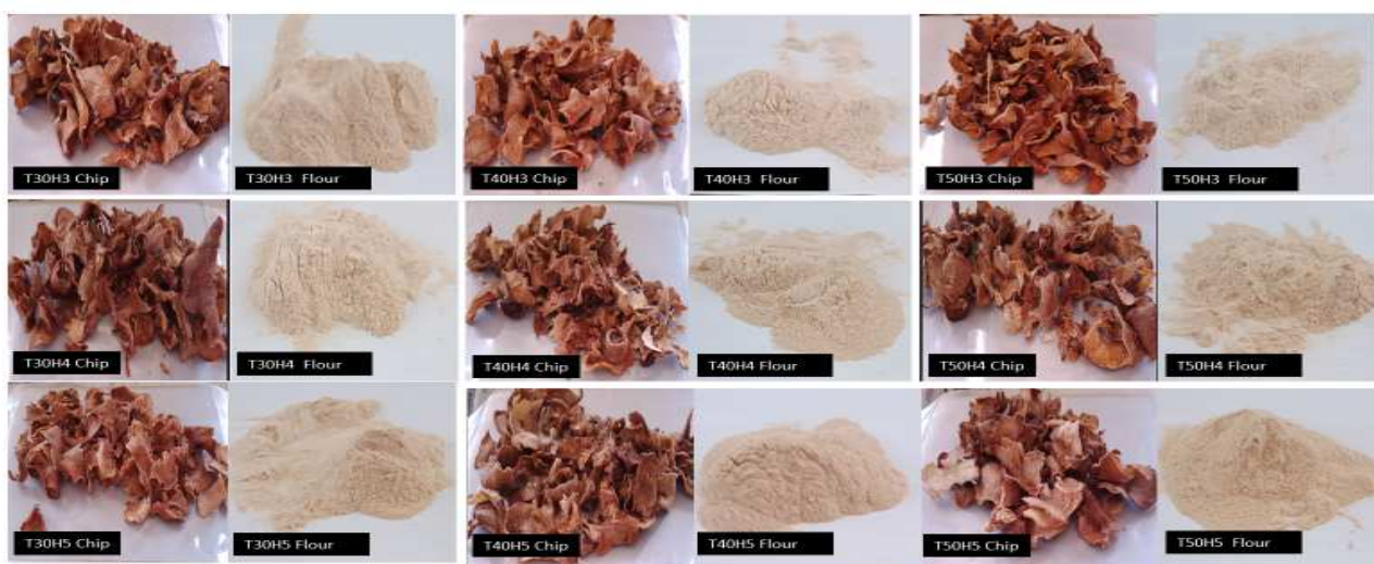
Fig. 1 Porang from different temperatures and times of annealing treatment in chip and flour form
