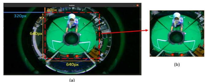
Fig. 3 Image cropping results. (a).Original image captured by camera. (b).Cropped image
