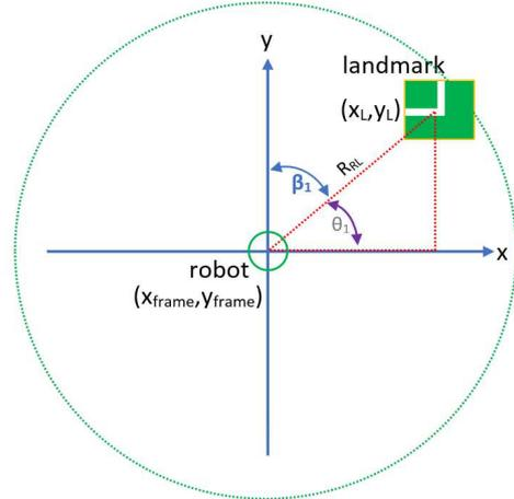
Fig. 8 View of landmark from camera with omnidirectional mirror perception
