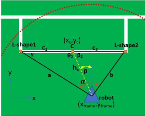
Fig. 9 Illustration to get robot orientation
