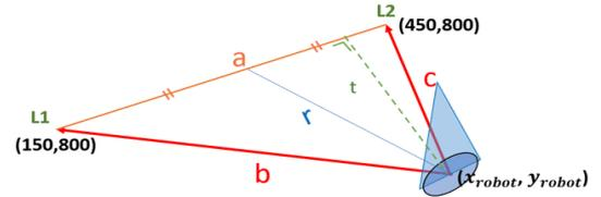
Fig. 11 Illustration of Robot Position Based on landmark
