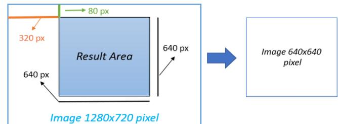
Fig. 2 Image cropping from 1280x720 to 640x640 pixel
