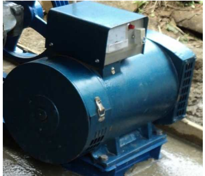
Fig. 10 ST-5 type synchronous generator
