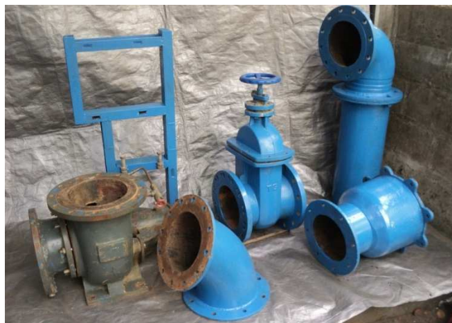
Fig. 9 Mechanical components of them from left to right: centrifugal pump, turbine/generator frame, elbow, gate valve, reducer, and draft tube
