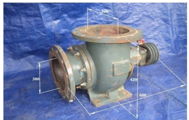
Fig. 8 10-inch centrifugal pump as the prime mover of the pico-hydro power plant
