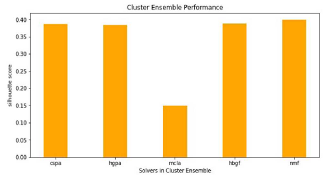
'cspa': Cluster-based Similarity Partitioning Algorithm. 'hgpa': HyperGraph Partitioning Algorithm. 'mcla': Meta-Clustering Algorithm. 'hbgf': Hybrid Bipartite Graph Formulation. 'nmf': NMF-based consensus clustering.
