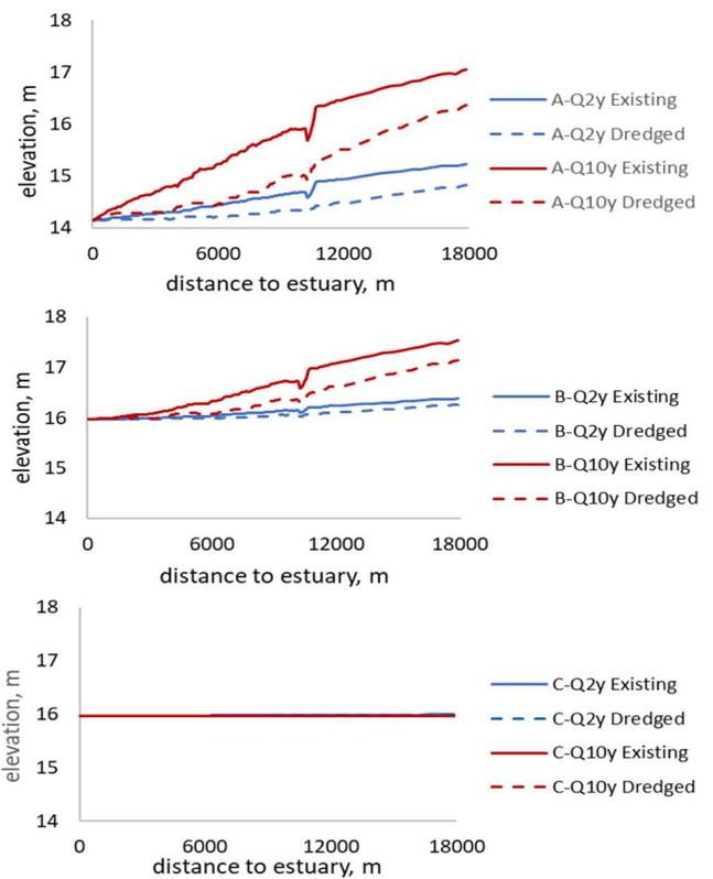
Fig. 9 Water level elevation of the Tulang Bawang River from 17.8 km to the estuary before and after dredging concerning 2 and 10-year return periods in boundary condition scenario A, B and C
