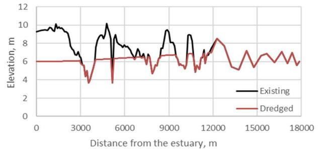
Fig. 6 Longitudinal cross-section of the riverbed in terms of the existing condition and dredging target
