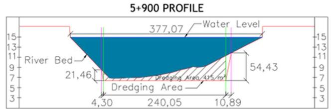
Fig. 4 Cross-section of the planned dredged section at a distance of 5.9 km from the estuary
