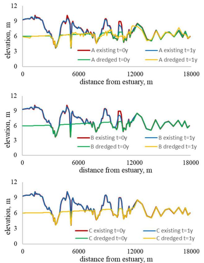
Fig 10 Riverbed elevation at existing and dredged conditions for scenarios A, B and C
