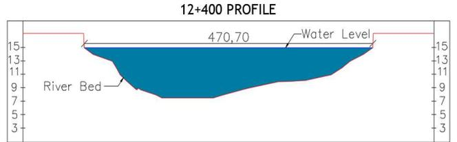
Fig. 5 Cross-section of the Tulang Bawang River along the stretch from 11.8 km (estuary) to 17.8 km (Dipasena) that is not considered to be dredged
