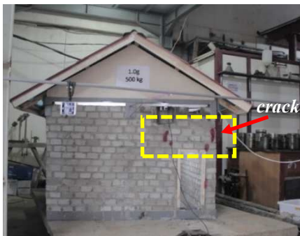
Fig. 18 Condition of the Front of the Specimen at the time of an earthquake acceleration of 1.0 g
