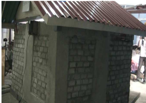
Fig. 26 Condition of the Right Side of the Specimen at the time of the 1.5 g earthquake acceleration
