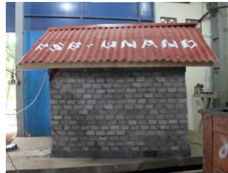
Fig. 19 Condition of the Left Side of the Specimen at the time of an earthquake acceleration of 1.0 g
