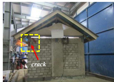
Fig. 24 Condition of the Back of the Specimen during an earthquake of 1.5 g
