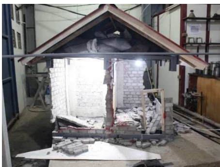
a. Condition of the Front of the Specimen during an earthquake acceleration of 1.5 g to Collapse.
