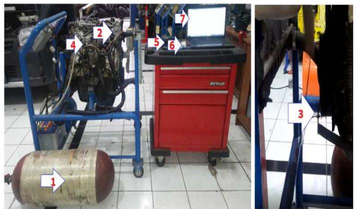
Fig. 4 Set up the engine speed data collection process and throttle valve position
