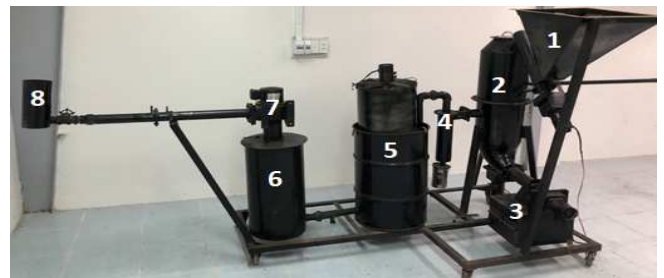
Fig. 1 The manufactured downdraft gasifier [11]
