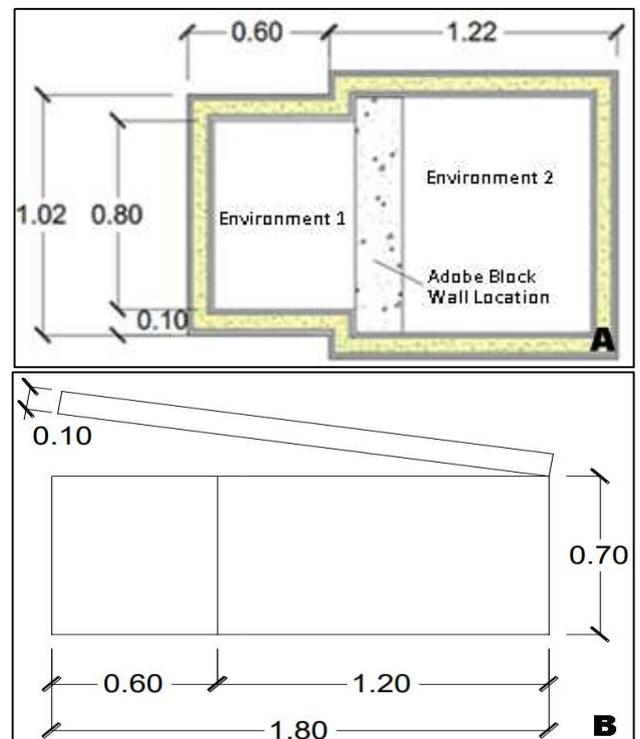
Fig. 4 Dimensions of the test chamber (A) Landscape view and (B) Side View
