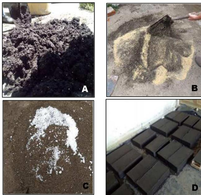
Fig. 1 (A)Sifted land, (B) Adding of sawdust, (C)Adding of EPS, (D) Adobe blocks molding
