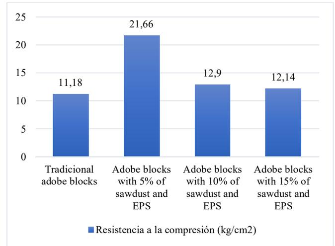
Fig. 3 Average compressive strength (kg/cm<sup>2</sup>) in blocks with different composition
