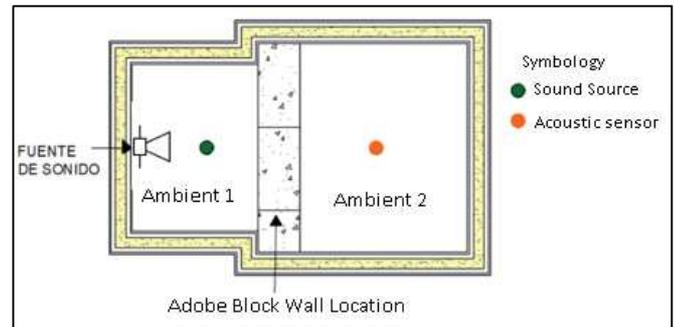
Fig. 9 Acoustic sensor location
