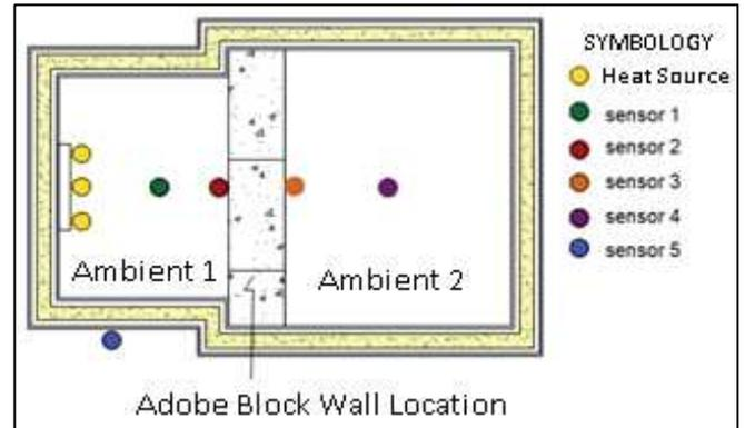
Fig. 7 Location of thermal sensors
