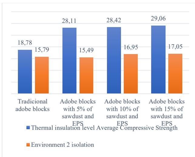
Fig. 8 Thermal insulation level in tested walls and Environment 2 isolation
