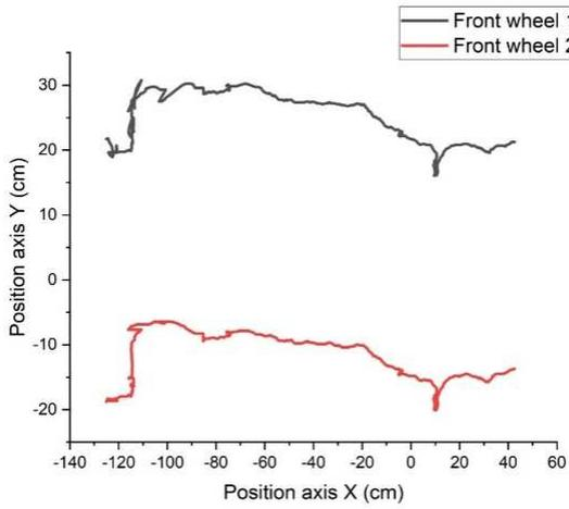
Fig. 7 X vs Y trajectory of the assistive device with the directional locking and anti-reverse systems activated
