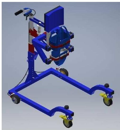
Fig. 2 Assistive device prototype, walker-type mechanism
