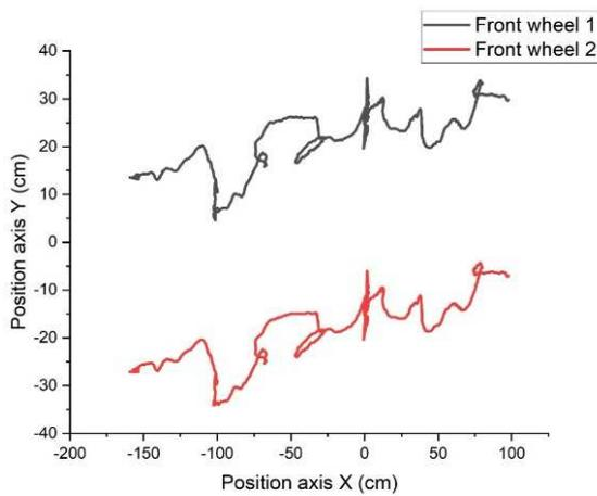
Fig. 8 X vs Y trajectory of the assistive device with the anti-reverse system deactivated
