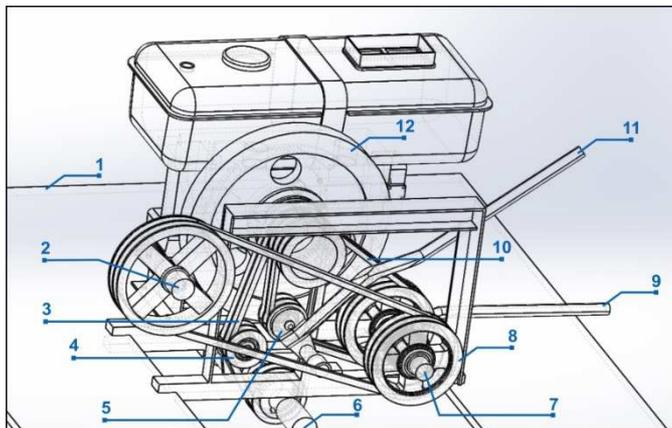
Fig. 3 Scheme of the transmission system in MRMU (1. Truck deck, 2. Polishing machine shaft, 3. Truck axle belt, 4. Fastening transportation belt, 5. Fastening milling machine belt, 6. Truck axle, 7. Rice milling shaft, 8. Rice milling pulley, 9. Fastening lever for rice milling, 10. Rice milling belt, 11. Fastening lever for transportation, 12. Flywheel).
