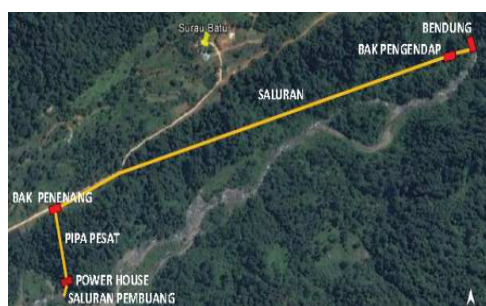
Fig. 9 Components of Microhydro power plant Andalas University
