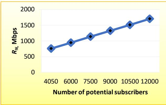
Fig. 10 The graph of the dependence of  $R_N$  on the number of potential subscribers
