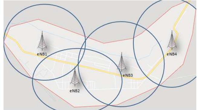
Fig. 12 The scheme of the LTE network in Muynak (with the geographical location of base stations)
