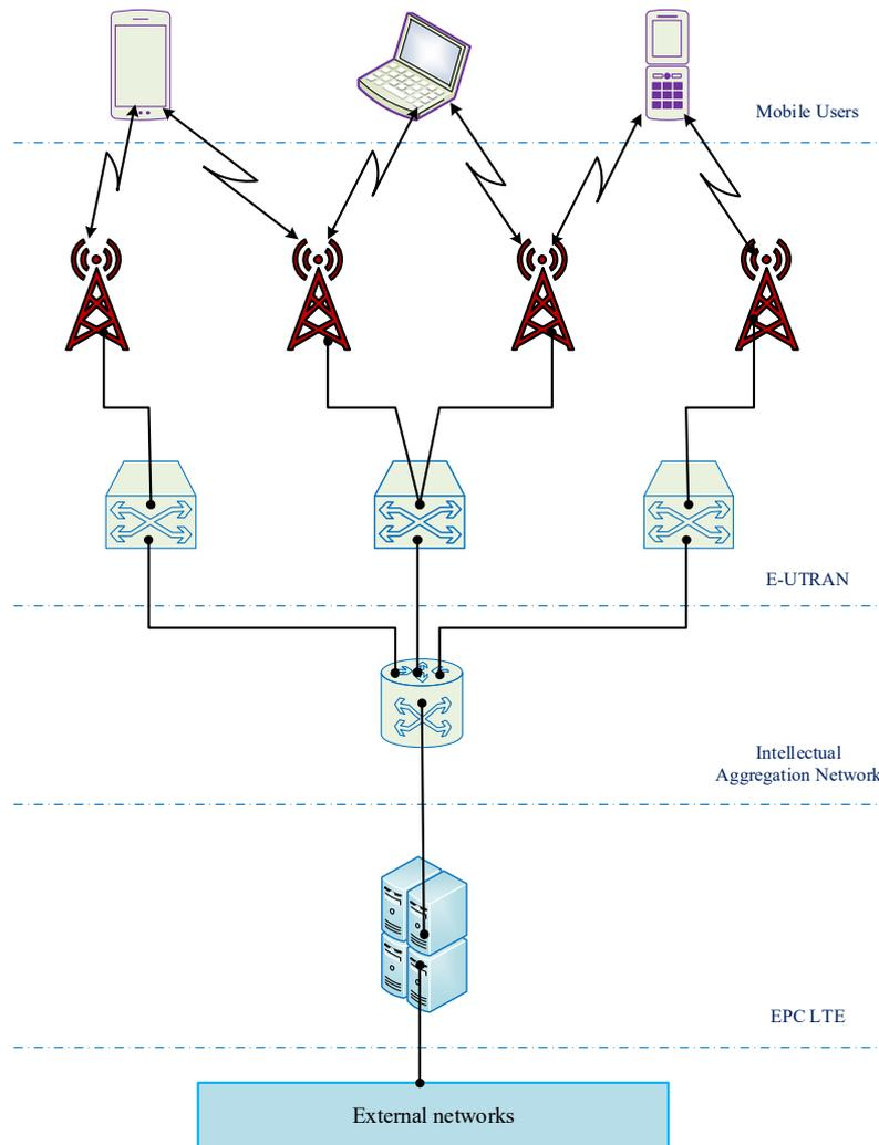
Fig. 13 The scheme of the LTE network in Muynak (with the geographical location of base stations)
