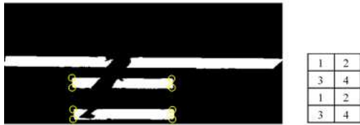
Fig. 7 Left: A binarized image with perspective distortion correction (yellow circles are added on vertices). Right: 2D label array representing the arrangement of vertices in the binarized image.
