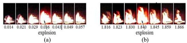
Fig. 13 The explosion flame of ceiba pentandra oil, (a) first explosion and (b) second explosion (s)
