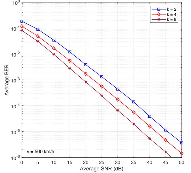
Fig. 6 The BER performances of FRMCS with  $K$  array-antenna element.
