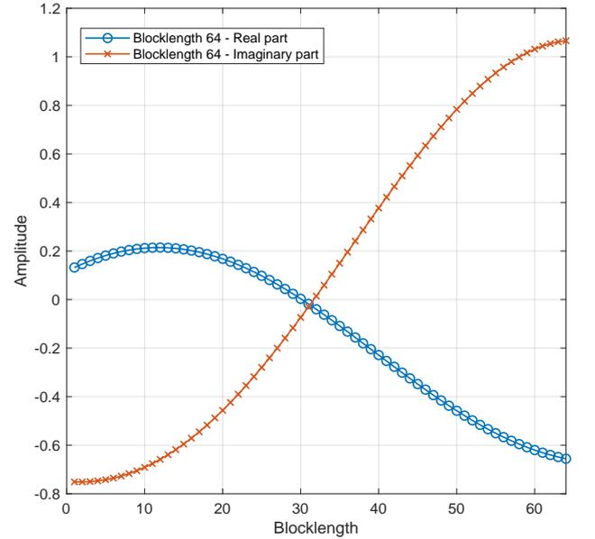
Fig. 9 The change of channels at  $f_d T_s = 0.5$  with blocklength 64.
