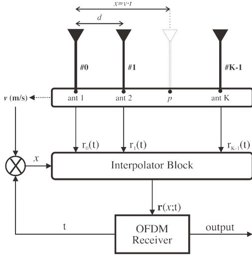
Fig. 3 The detailed structure of the proposed array antenna-assisted DSC.
