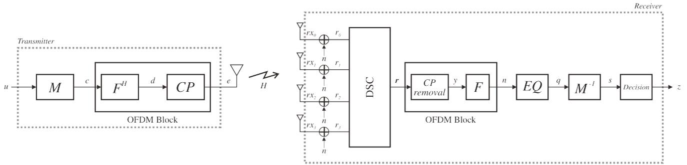
Fig. 1 Transmission structure of FRMCS using the proposed DSC.
