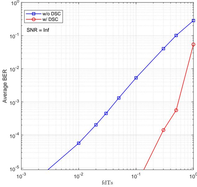
Fig. 7 The BER performances of FRMCS with and without DSC at different  $f_d T_s$ .
