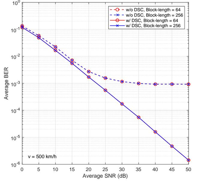
Fig. 8 Performances of FRMCS with and without DSC showing that the performance is not affected by the blocklength due to the normalized Doppler.
