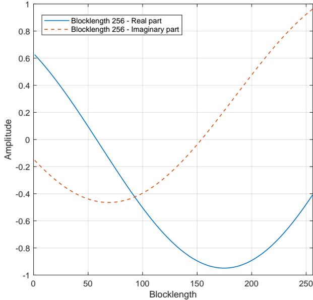
Fig. 10 The change of the channels at  $f_d T_s = 0.5$  with blocklength 256.
