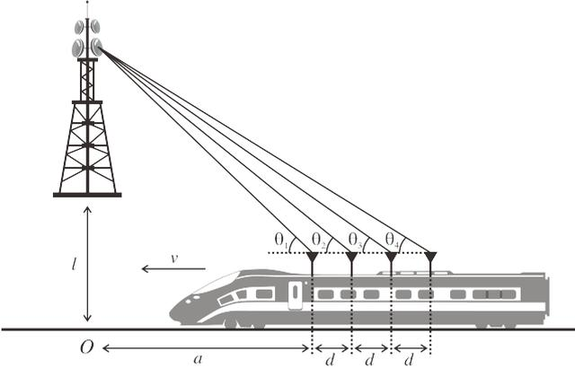
Fig. 2 The proposed array antenna-assisted DSC for FRMCS.
