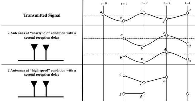
Fig. 4 Effect of Doppler spread experienced by each antenna element.
