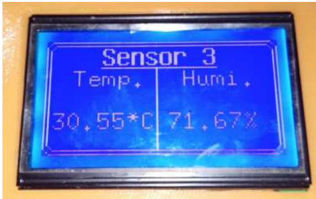
Fig. 6 Display of temperature and humidity data on the GLCD
