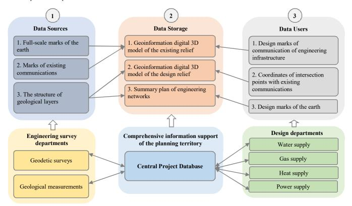
Fig. 4 BIM-structure of Central Project Database
