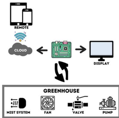
Fig. 3 Diagram of Smart Greenhouse Automation System
