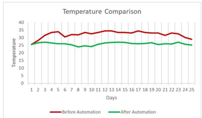
Fig. 6 Comparison between Smart Greenhouse Temperature and Outside Greenhouse Temperature
