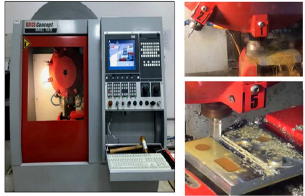
Fig. 5 Machining of sample component using CNC 3axis vertical milling machine monitored by IoT device
