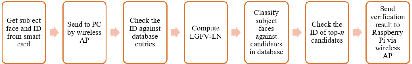
Fig. 4 The process of verifying a person using the proposed mobile face verification system
