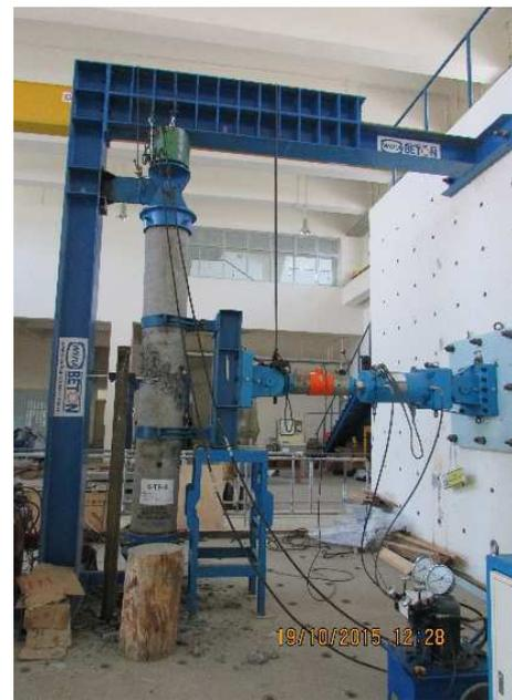
Fig. 5 Test setup of specimen and loading system for cyclic flexural with axial load testing
