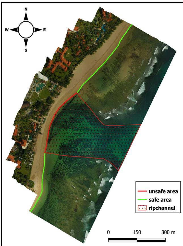
Fig. 12 Surf zone mapping from UAV-orthophoto.
