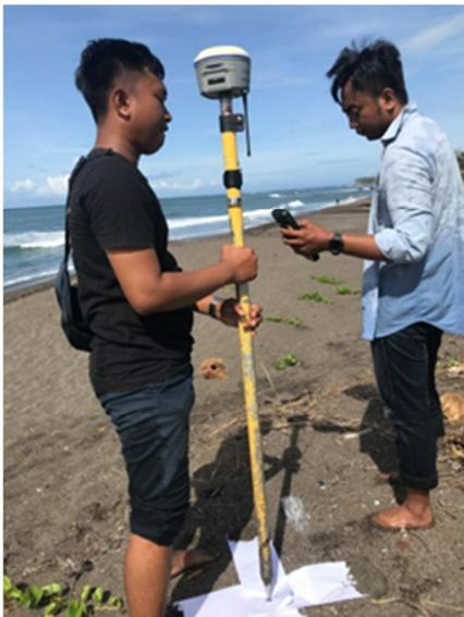
Fig. 7 Measurement of GCP coordinates
