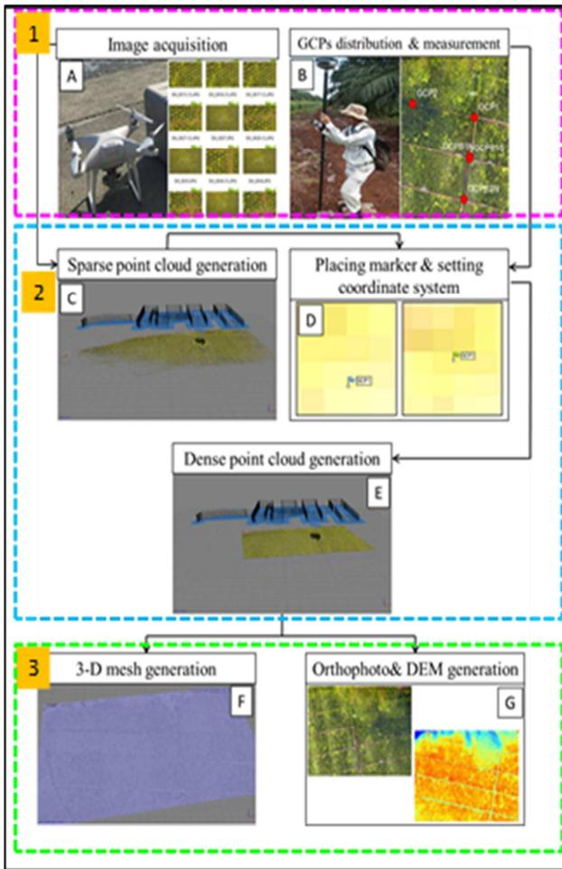
Fig. 9 Workflow of making orthophoto and DSM
