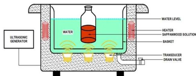
Fig. 2 Schematic representation of ultrasound-assisted extraction of antioxidant compounds from sappanwood.
