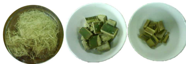
Fig. 1 Bamboo samples used as raw material: dried bamboo fiber (left), wet bamboo chip (middle), and dried bamboo chip (right).
