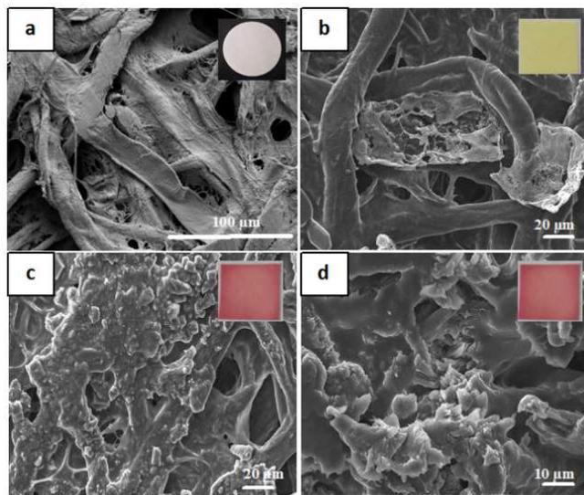
Fig. 6 SEM images of filter paper (a), curcumin paper strip surface (b), curcumin paper strip-boric acid surface (c) curcumin paper strip-boric acid, cross section (d)
