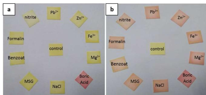
Fig. 7 Detection of curcumin paper strip towards 10000 ppm of various sole chemicals (a), chemicals + boric acid mixture (b).
