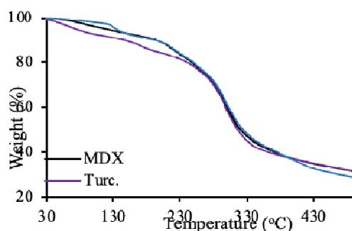
Fig. 1 TGA curve of of turmeric, maltodexktrin and maltodextrin-ethanolic curcumin extract
