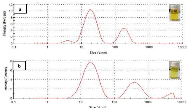
Fig. 2 Curve of particle size distribution for CURNns (a), and CURNnsr (b)
