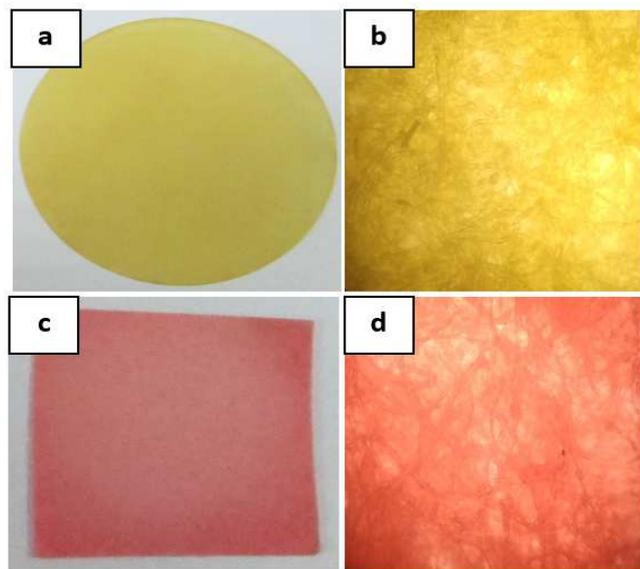
Fig. 5 Appearance of curcumin paper strip (a), optical microscope image of curcumin paper strip (b), curcumin paper strip upon contact with boric acid (c), optical microscope image of curcumin strip-boric acid (d)
