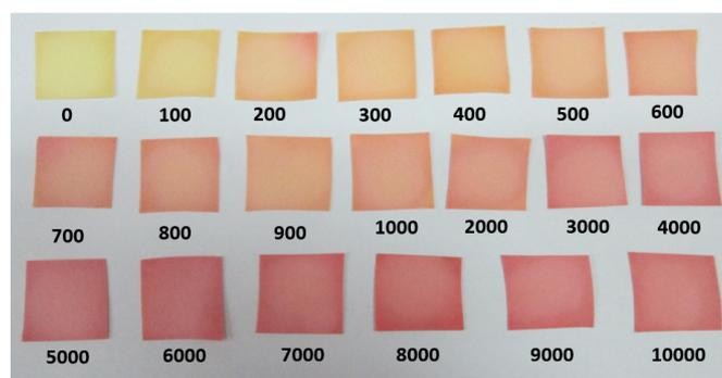
Fig. 8 Color scale of the curcumin paper strip response to various concentration of boric acid solution from 100-10000 ppm
