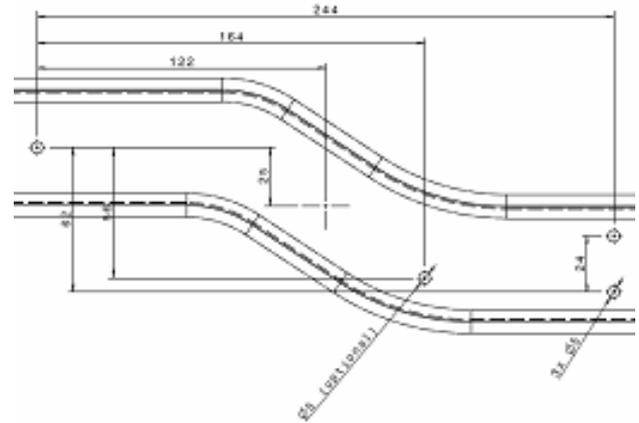
Fig 2. S-Rail model hole dimensions in mm.
