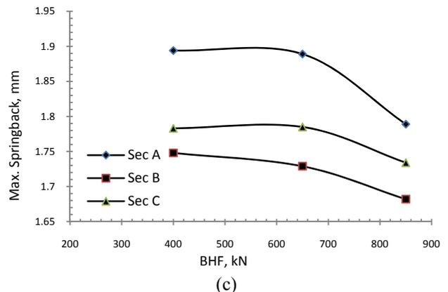
Fig. 8 Maximum springback error prediction on section A, B and C, (a) No drawbead, (b) Smooth drawbead and (c) Locking drawbead
