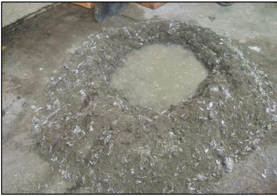
Fig. 8 Mixture of mortar and polypropylene fiber
