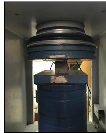
Fig. 6 Compressive test on mortar
