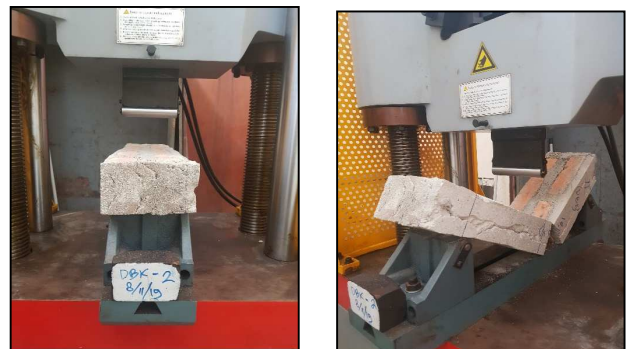
Fig. 12 Flexural test of DBP
