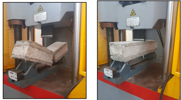
Fig. 11 Flexural test of DBPP
