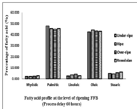
Fig. 5c. Relationship of the ripening levels of FFBs and processing delay times of 60 h with the profile of palm oil fatty acids.
