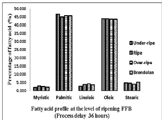
Fig. 5b. Relationship of the ripening levels of FFBs and processing delay times of 36 h with the profile of palm oil fatty acids.
