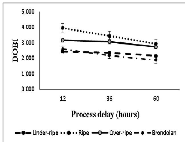
Fig. 1. Relationship of DOBI values with the processing delay and ripening level of FFBs.
