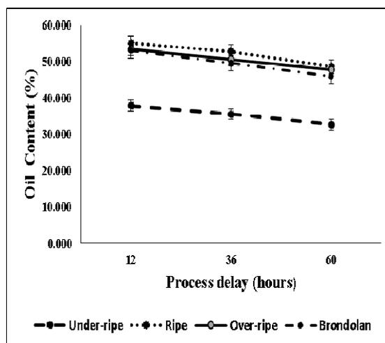
Fig. 4. Relationship of oil content with the processing delay and ripening level of FFBS.
