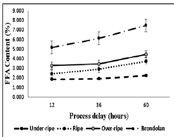
Fig. 2. Relationship of FFA content with the processing delay and ripening level of FFBS.
