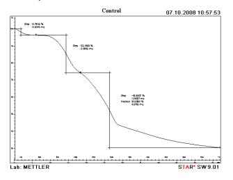
Fig. 5 Thermogravimetric analysis curve for the control sample
