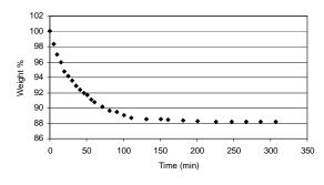
Fig. 3 Weight loss versus time for drying at 60°C.
