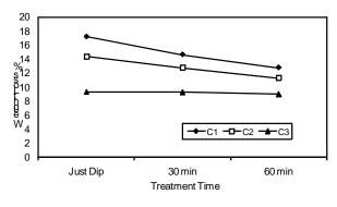
Fig. 4 Flammability results for different fire retardant concentrations at different dip time
