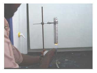
Fig. 1 Flamability test using the vertical burning column
