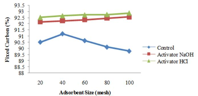
Fig. 5 Effect size and type activators adsorbent against fixed carbon on adsorbent ACHJ
