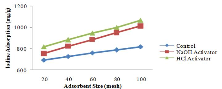
Fig. 6 Effect size and type activators adsorbent against iodine adsorption in adsorbent ACHJ
