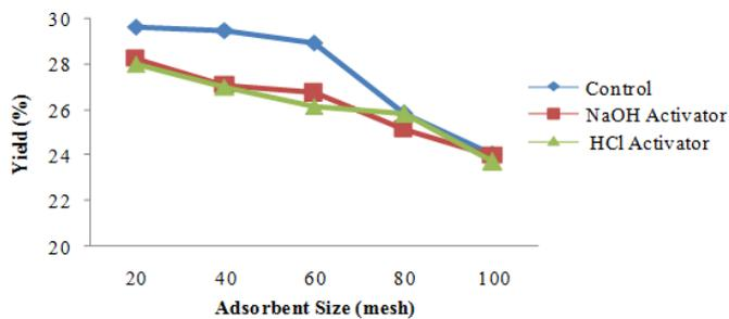
Fig. 1 Effect of adsorbent size and type activators adsorbent against yield on adsorbent ACHJ
