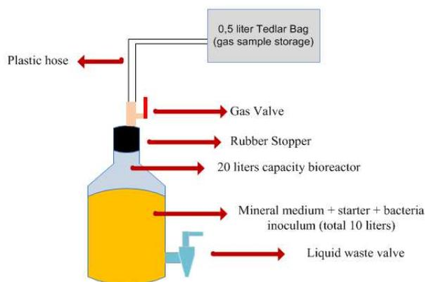
Fig. 1. Bioreactor Set-Up
